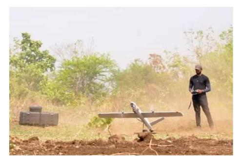
Armed with a 1 kg high-explosive fragmenting warhead designed to neutralise soft-skin targets, the UAV is also equipped with day and night surveillance cameras for round-the-clock intelligence gathering. Unique among its class, the system allows for mission abort, in-flight recovery, and reuse via a parachute recovery mechanism.
