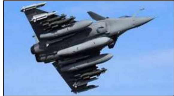
A fully loaded Rafale fighter with Hammer, SCALP and Meteor air-to-air missile and munitions.
