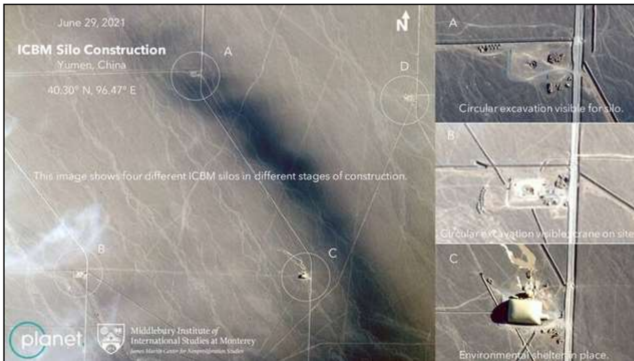
This image shows four different ICBM silos in different stages of construction. (Credit: Planet Labs Inc)
