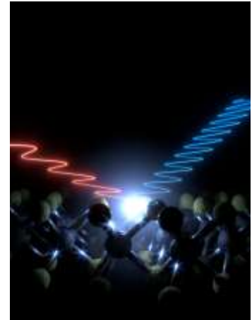
A red laser beam impinges on the atomically thin crystal WSe 2 , which converts the red light of the laser into a blue glow. Credit: Felix Hofmann
