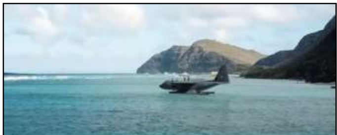
A rendering of an amphibious modification to an MC-130J Commando II. US Air Force Special Operations Command
