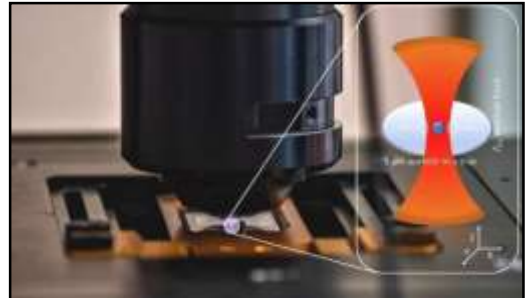
A microparticle held with optical tweezers in the microscope. Inset: Illustration of the held particle (magnified); shown in red is the light of the infrared laser used. Credit: Pascal Runde
