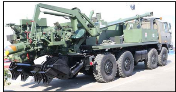
The Ordnance Factory Board has developed a 155mm truck-mounted howitzer. (Gordon Arthur)
