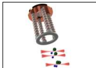
To shield the molecules, they are exposed to microwaves from an array of antennas. Credit: Radboud University
