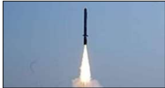
Nirbhay is a subsonic missile, flying at a speed of 0.7 Mach.
