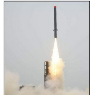
A new version of the subsonic cruise missile Nirbhay as seen here, will be test fired with short turbo fan engine and an advanced radio frequency seeker. (Photo | EPS)
