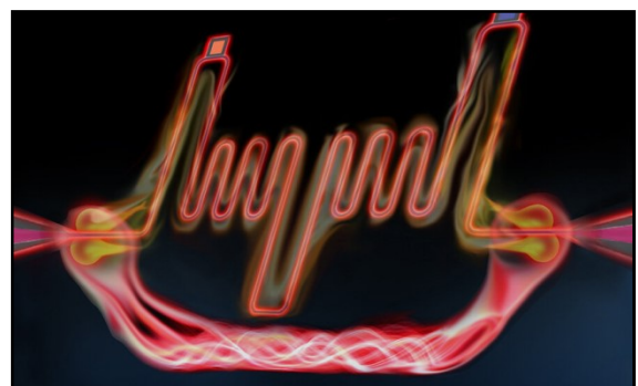
Entangled pairs of photons are generated by and propagate away from qubits placed along a waveguide. Credit: Sampson Wilcox
