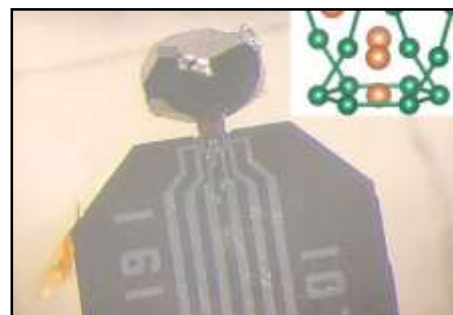
A small crystal of the new material, a synthesis of Niobium and Germanium ( \text{NbGe}_2 ), is mounted on a device to examine the behavior of the new electron-phonon liquid. The inset shows the atomic arrangement in the material. Credit: Fazel Tafti, Boston College
