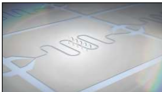
Researchers at Argonne have demonstrated an on-chip quantum circuit and realized strong coupling between a superconducting resonator and a magnetic device. This earlier research introduced a new platform for investigating quantum information processing. Credit: Ellen Weiss/Argonne National Laboratory.
