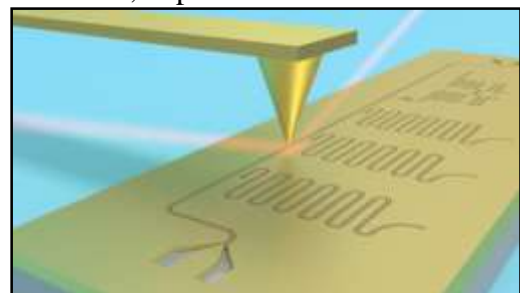
Schematic of a superconducting circuit being imaged using terahertz scanning near-field microscopy. Credit: The University of Queensland
