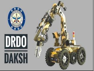
The Remotely Operated Vehicle can be controlled either by wireless communication over 500m line of sight or by fibre optic communication over 100m distance. It can work continuously for 3 hours in just a single recharge.
