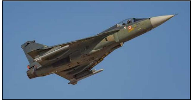
With a top speed of Mach 1.6 to 1.8, a maximum external load of 7,700 pounds and a service ceiling of fifty-two thousand feet, the Tejas remains unexceptional compared to top-performing fourth-generation light fighters such as the F-16. The Indian Air Force has only ordered 123 Tejas jets so far to equip six squadrons by 2024. HAL, however, is having difficulty ramping up production from eight aircraft a year to the desired sixteen.
