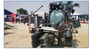
DRDO scientist Alok Mukherjee said, "These robots are controlled remotely from a distance of 2 km. The operator can locate and defuse the explosive by using high pressure water jets." Alok Mukherjee has been part of the developing team of this Unexploded Ordnance Handling Robot (UXOR).
