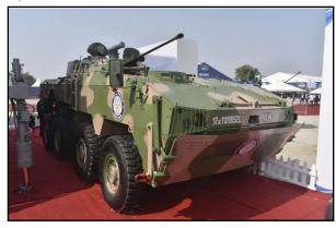
varying between 19 and 26 tonnes, with amphibious capability provided at up to 24 tonnes. The WhAP, which can reach a top speed of 100 km/h on land, has a cruising range of up to 500 km.
