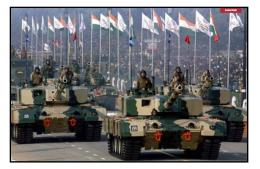
the state-run Defence Research and Development Organisation (DRDO) was tasked with developing the tank. It was to be a forty-ton vehicle, armed with a 105-millimeter gun. It would be small enough to be strategically mobile, capable of being shuttled on internal lines (roads and railroads) to vital sectors along the long border with Pakistan.
