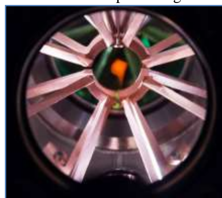
Ultracold atomic cloud of rubidium atoms used in this experiment: You can see the fluorescence that occurs during laser cooling. Credit: AG Ott/TUK
