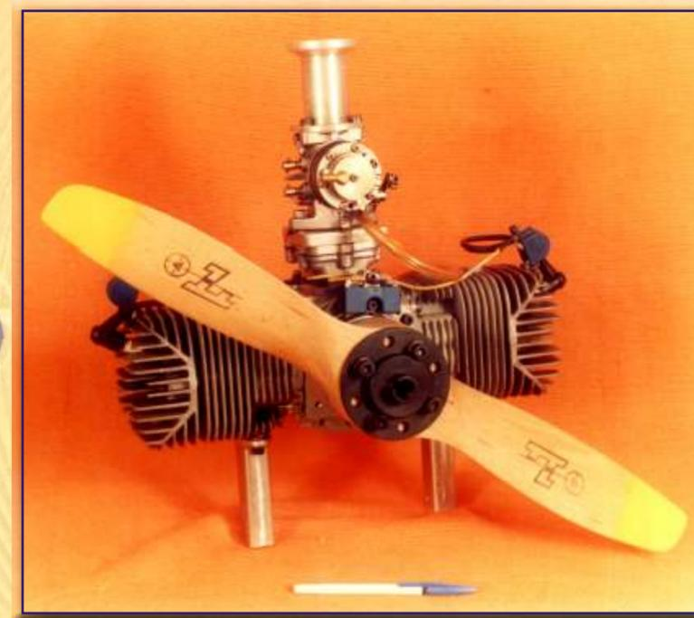
Two cylinder engine for UAV
