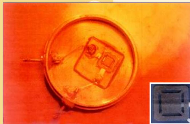
Bonded and packaged vibration sensor. Inset: sensor chip
