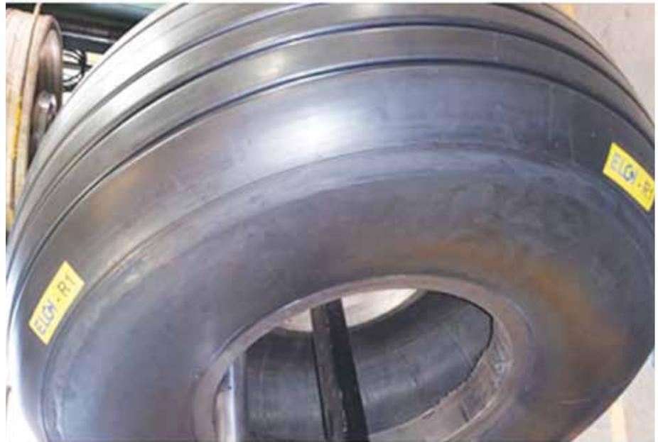
higher number of landings as compared to the new foreign tyre (132 landings compared to 80 landings). This significant achievement has translated in to supply of retreaded tyres to the IAF. Process of flight trials after second retread is already in progress at an IAF base. Aviation
