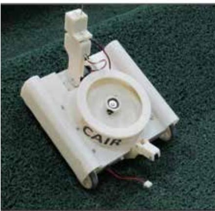
The wall climbing robot is a miniature tracked robot capable of climbing vertical walls. It uses an impeller to
