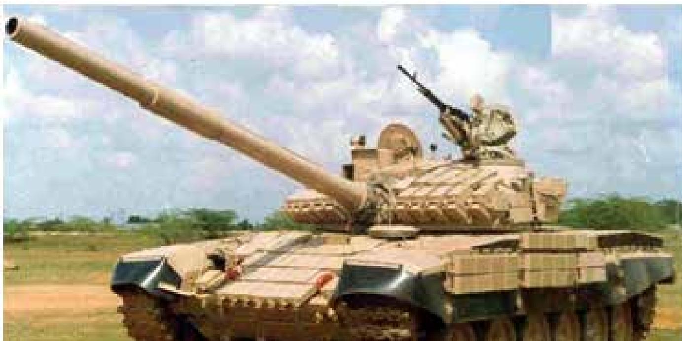
and PXE as project partners. HEMRL has developed the reactive elements, DMRL carried out development of armour materials for panels and CVRDE has finalised the layout and fitment of panels on tank T-72 and Arjun Mk-II. PXE provided the experimental facilities for dynamic evaluation of ERA Mk-II panels against 125 mm FSAPDS ammunition.
