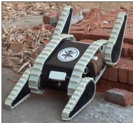
The Miniature Unmanned Ground Vehicle (MINIUGV) uses tracked locomotion to negotiate rough terrain and features found in a typical urban terrain including steps and staircases. It is a remotely-controlled man-portable robot which can be used for surveillance and reconnaissance in low intensity conflict operations.
