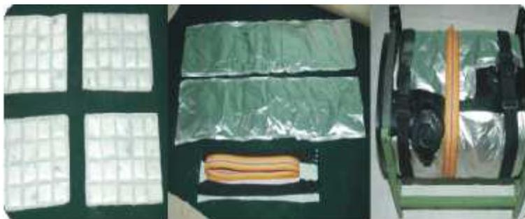
Left to right: Heating pouch; Al foil bag containing heating pouch; and heating pad wrapped around diesel tank
