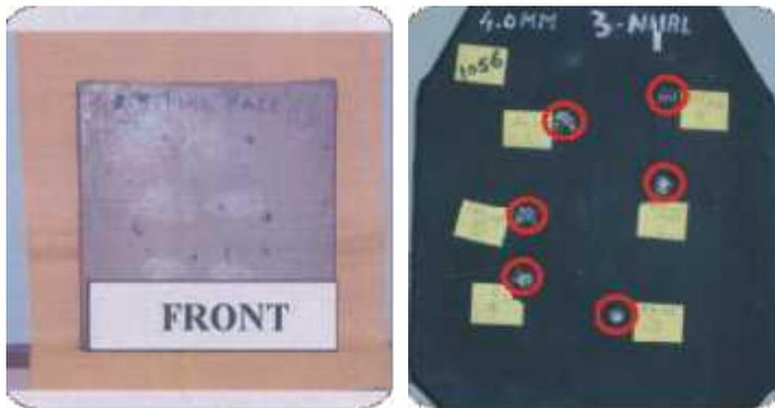
ZTA composite body and vehicle armour before (left) and after ballistic testing (right)
