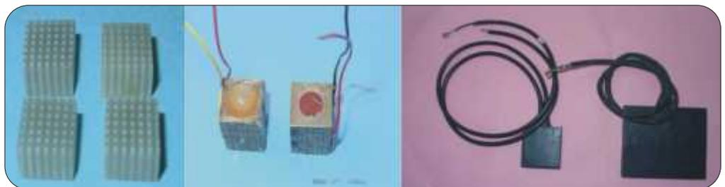
Left to right: Piezocomposite transducer elements, 4-element piezocomposite stacks, and piezocomposite hydrophones
