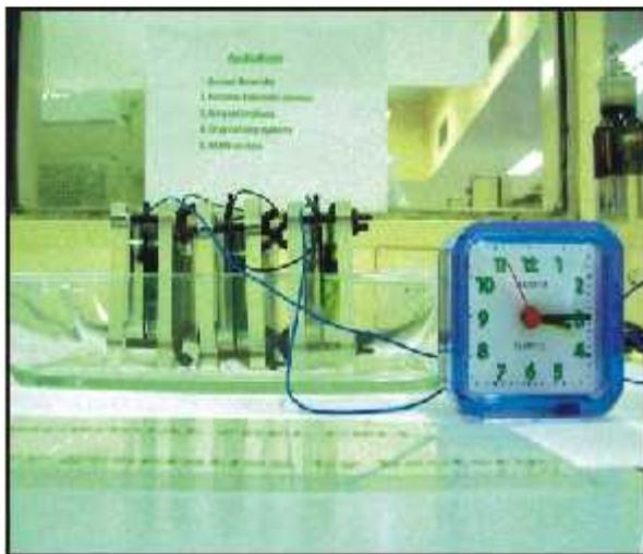
Clock running on microbial fuel cell based on anaerobic bacterium *Desulfovibrio* sp.
