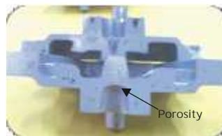
Porosity in liquid die cast component
