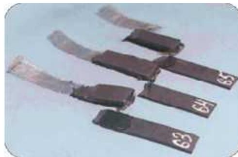
Failure pattern of rubber adhesive to metal using PU sealant
