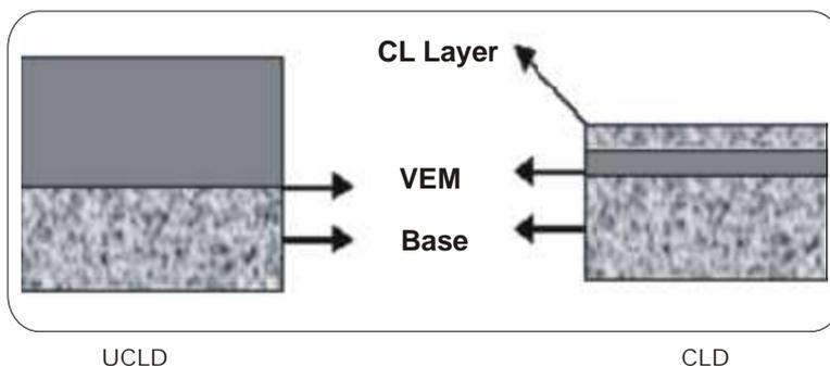
UCLD and CLD systems for various metallic and composite structures have been developed and extensively evaluated for the various substrates. The elastomeric material of these systems is especially designed to damp vibrations in wide frequency range when applied on mild steel, aluminium or FRP composites. Material and application technology for each vibration case has been studied and standardised.
