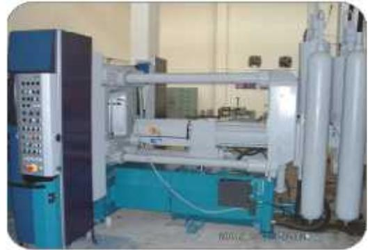
Cold chamber high-pressure die casting machine
