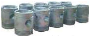
SSM cast A356 thick section pistons
