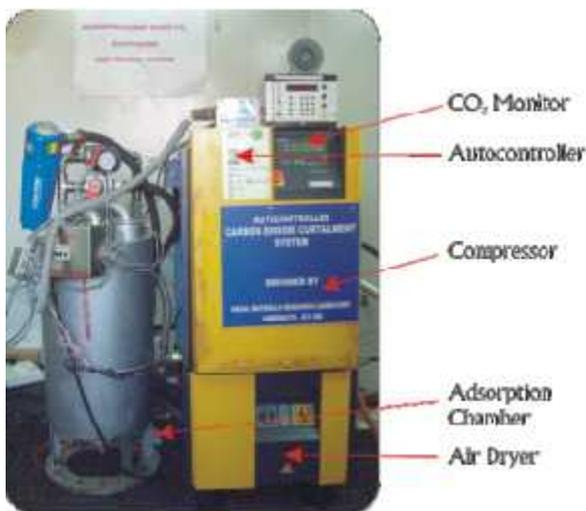
Autocontrolled CO<sub>2</sub> system
