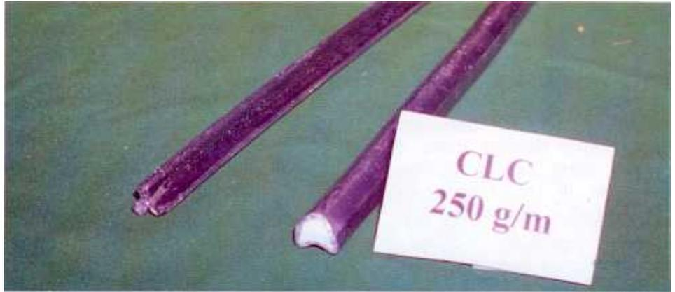
250 g/m flexible linear shaped charge
