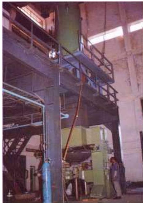
500 tonne capacity *Ti* sponge ejection press
