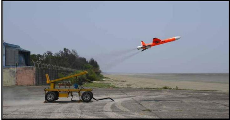
During the recent trial, it EW for 32 minutes and successfully cleared 21 way-point-navigation modes. The MEMS based (Micro-Electro-Mechanical Systems) navigation developed by RCI Hyderabad came to its rescue this time.
