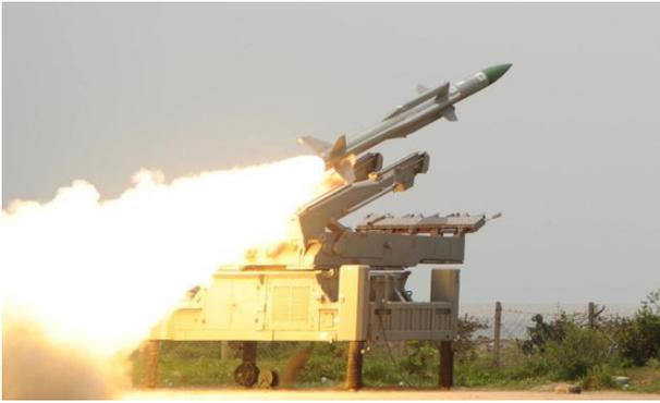
**4. Akash:** - Akash missile is a medium range surface to air missile. It was successfully launched in 1990 for the first time. It has an intercept range of 30 kms. It has an inbuilt radar system which is used to intercept not only fighter jets but can also neutralise the cruise missiles.
