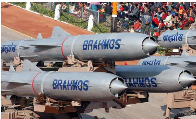
**3. BrahMos:** - This missile is named after Indian river Brahmaputra and Russian river Moskva. It is a short-range supersonic cruise missile. The missile has three variants: land based, naval based and air and submarine based. BrahMos was first test-fired in 2001 from the Integrated Test Range (ITR), Chandipur. It has an operational range between 290 and 300 kms.
