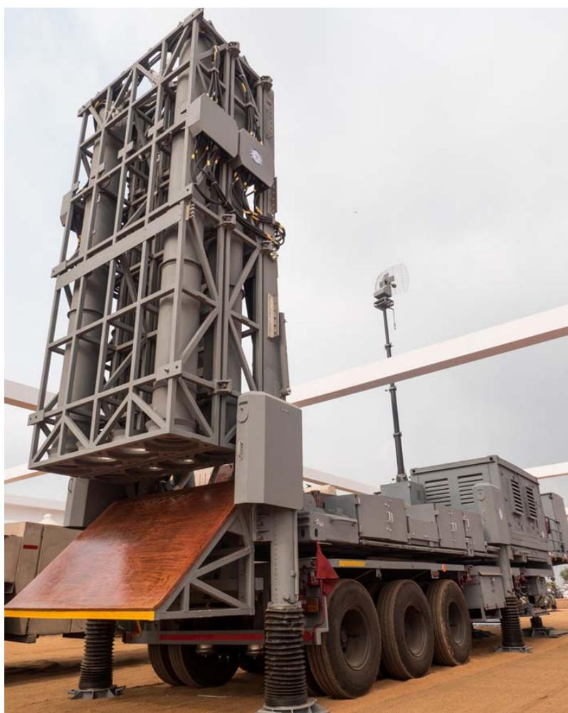
**The MRSAM fire unit holds eight ready to launch missiles in two stacks. The missiles are fired vertically from their canister-launchers. To protect the fire unit assembly DRDO developed a unique thermally protected flame deflector that directs the rocket flames away from the trailer. This heat deflector can endure at least 60 launches, without damage. Photo: Noam Eshel, Defense-Update**
