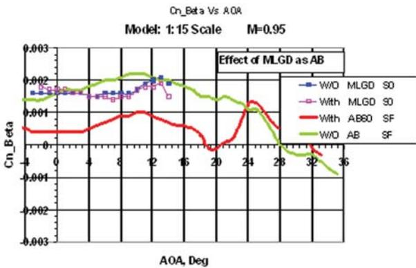
Figure 12.  $C_{n\beta}$  with MLG door.
