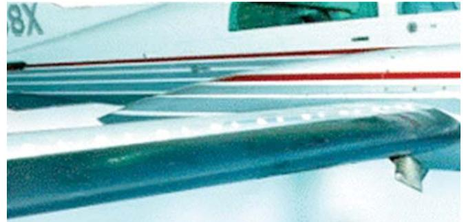
Figure 3. Vortex generators in wing.
