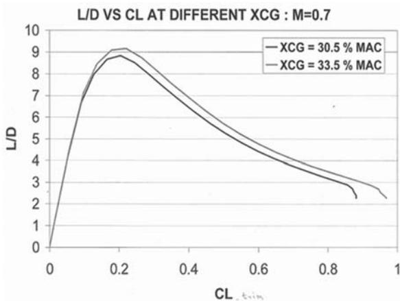
Figure 21. L/D for forward and aft C.G condition.
