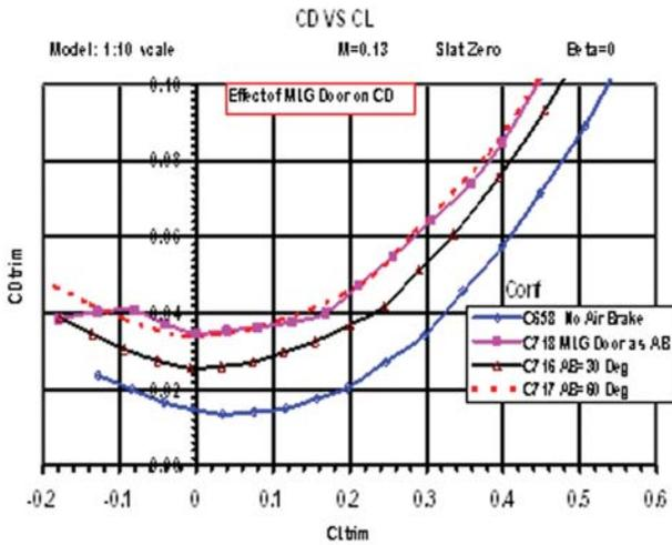
Figure 11. Drag coefficient with MLG door..
