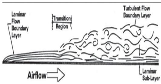
Figure 2. Boundary layer in a flat plate.
