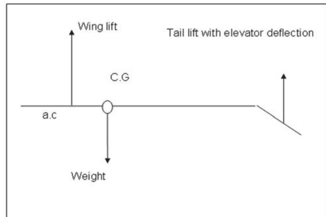
Figure 7. Unstable aircraft force balance.
