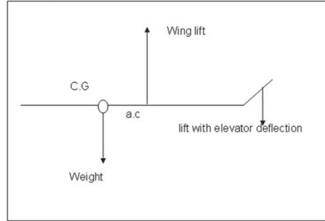
Figure 6. Stable aircraft force balance.
