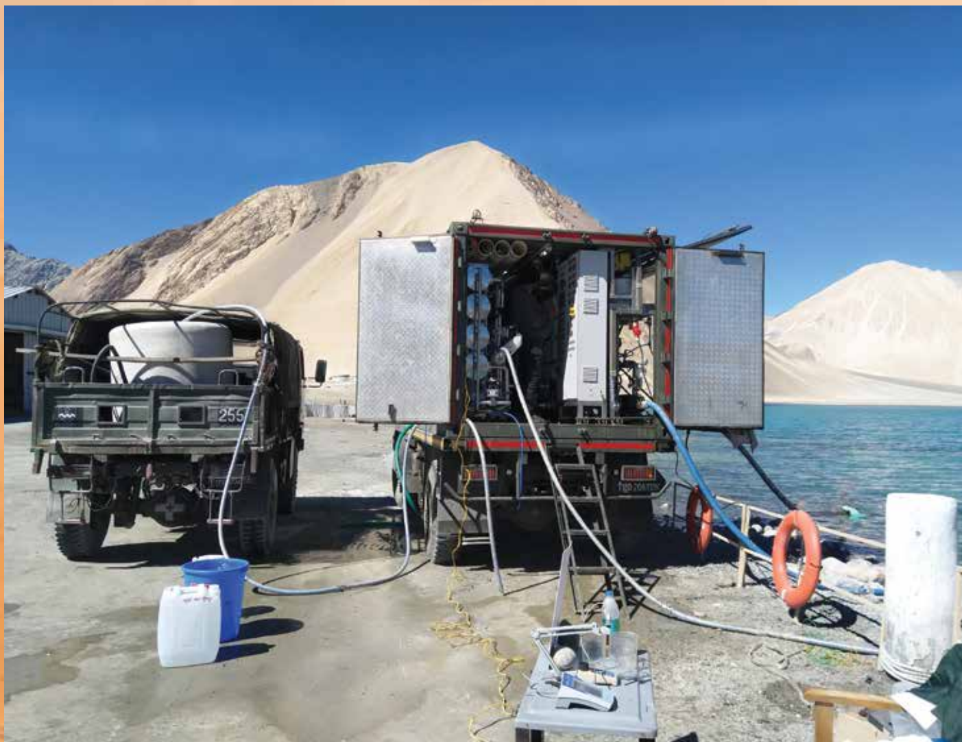
Chemical, Biological, Radiological, and Nuclear Water Purification System (CBRN-WPS) deployed at Lukung, Pengong Lake, Leh-Laddakh
