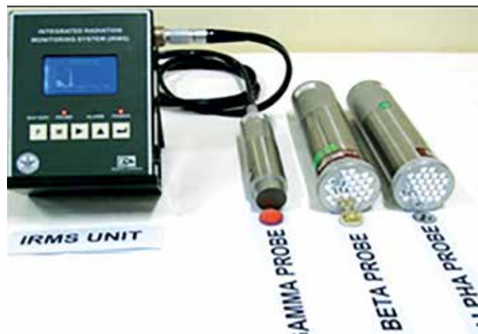
Integrated Radiation Monitoring System
