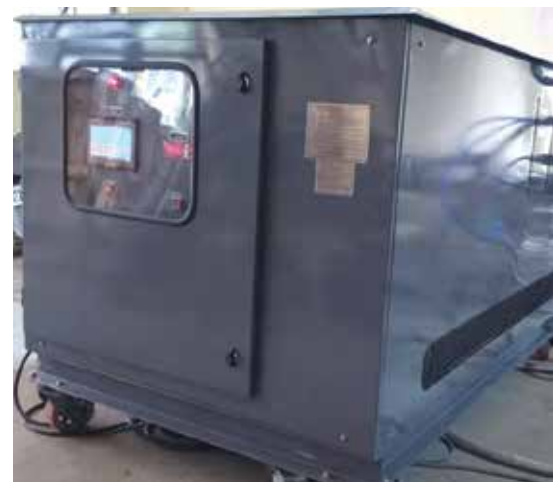
Latent Heat Storage based Thermal Management Unit for High Energy Laser-based DEW System
