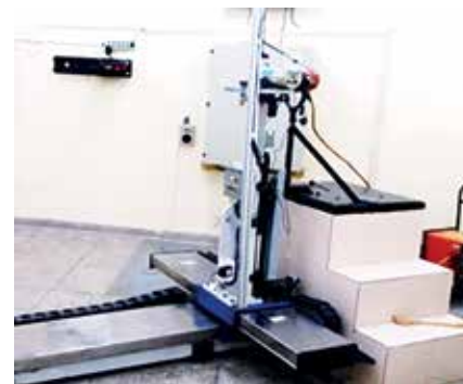
Positioning System of Medium Gamma Exposure Facility
