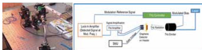
Fig 51. (a) Testing of THz Modulator by Optical Pumping (b) Schematic for Testing THz Detector
