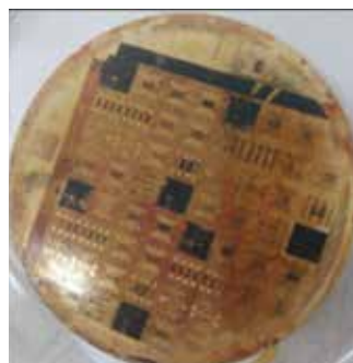
Fig 28 (a) Image of 2 inch Alumina Membrane with 50 Device Arrays
