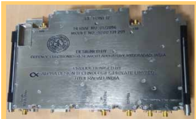
Single Channel as RF Tuner (0.5-18 GHz)
