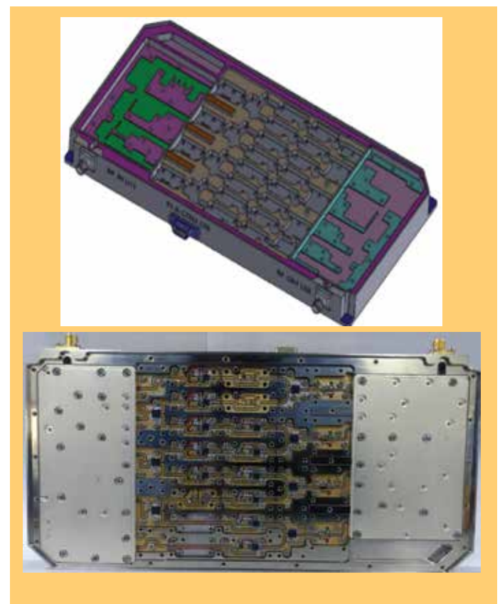
3-D Solid Model and Realised Switch Multiplexer Unit
