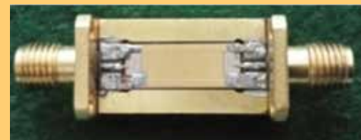
Filter 2.75-3.25 GHz 14.4 X 5.9 X 1.6 mm 3
