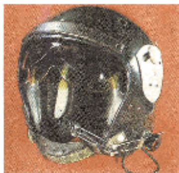
Fig. 35 Helmet made from glass-sisal-polyester/epoxy composite
