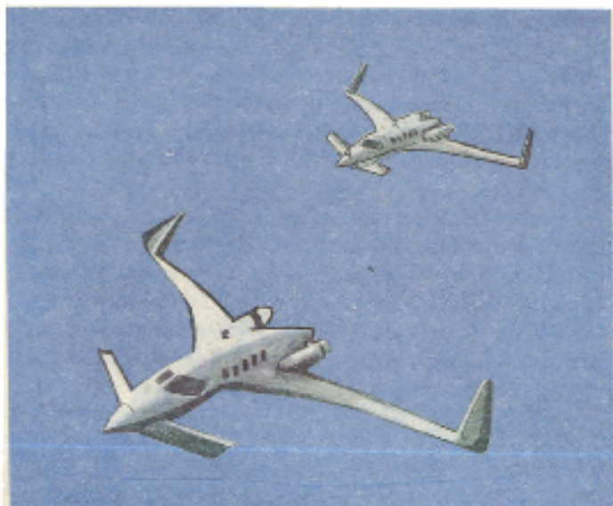
Fig. 7 All-composite starship 1 business aircraft produced by a subsidiary of Maytheon Company
