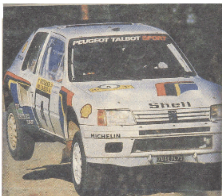
Fig. 15 Peugeot car (model 205) fabricated from aramid and carbon fibre-epoxy composite
