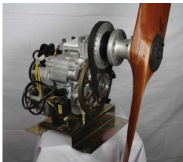
55 HP Rotary engine
