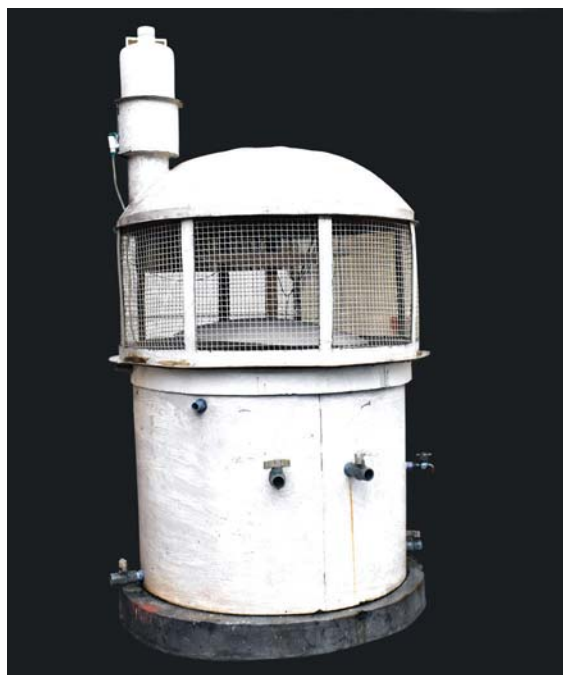
Iron Removal Unit
