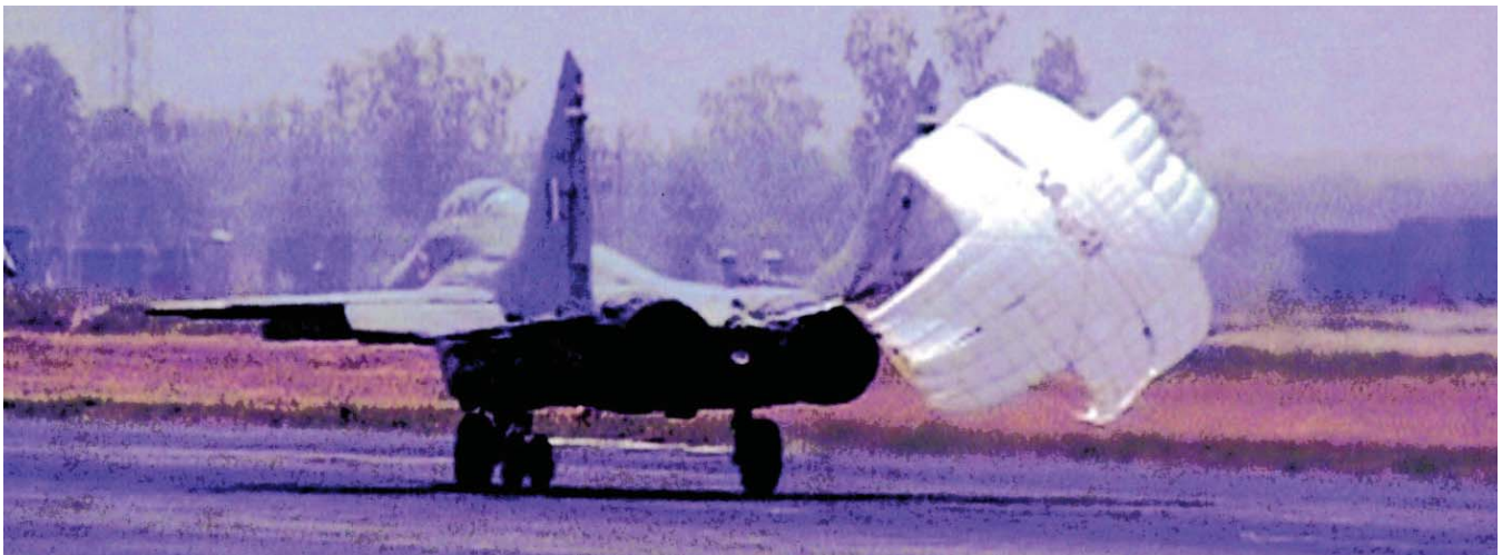
Brake Parachute for MiG-29 Aircraft
