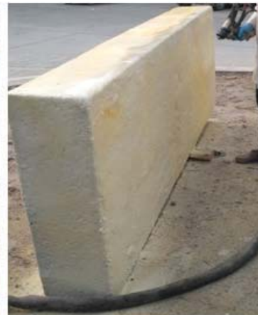
Polyurea coated concrete Slab
