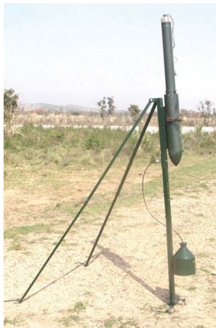
Bund Blasting Device
