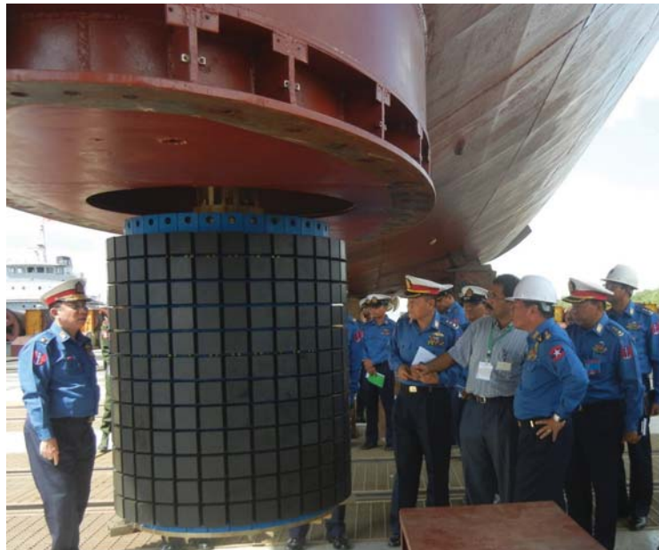
HMS-X Array Onboard a destroyer class ship
