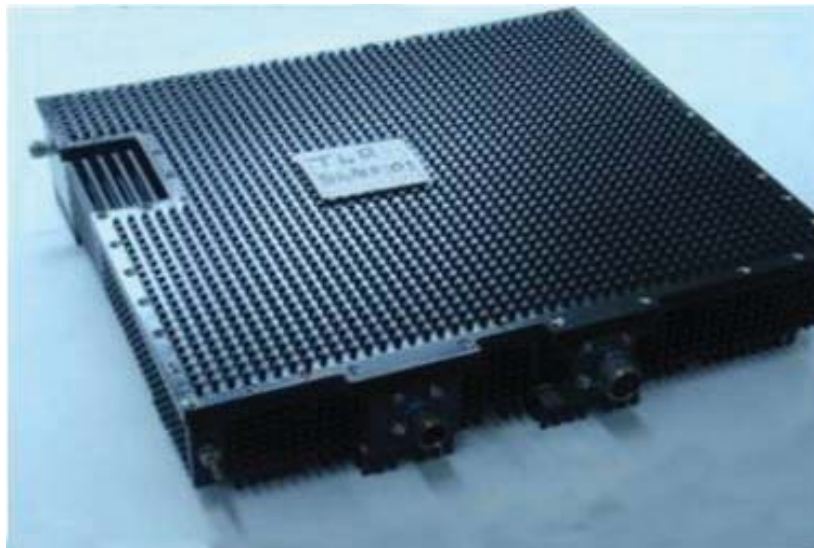
120W Pulsed X band Microwave Power Module
