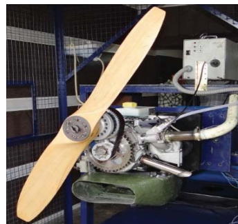
65 HP Rotary engine
