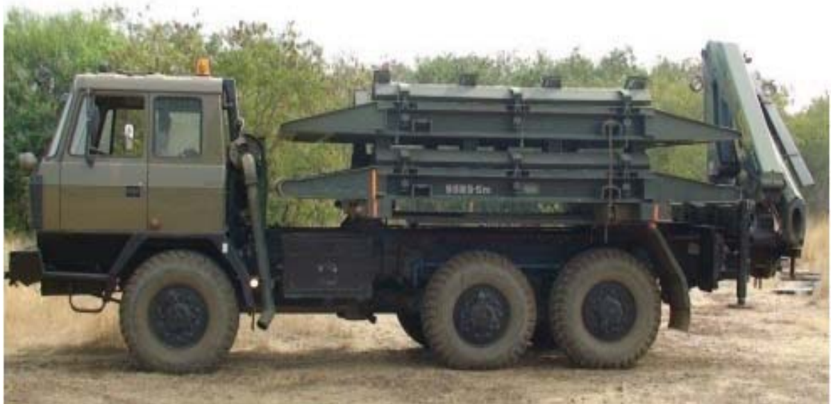
5m Short Span Bridging System
